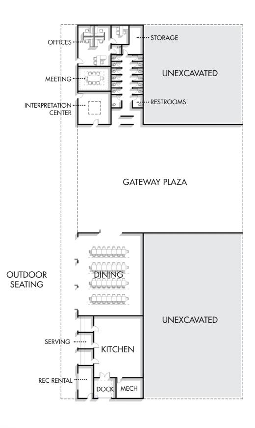
EMBEDDED IN THE LANDSCAPE / The building is embedded in the ground allowing the bike path to pass above the pedestrian traffic to mitigate site circulation congestion. The green-roof of the building minimizes storm-water run-off on the site
