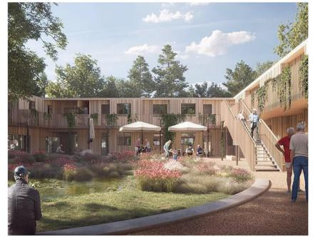
The material character is defined by an extensive use of wood, and sets a warm and natural tone that will only improve with age. The structure is built with Cross Laminated Timber (CLT) which enhances the sustainability of the project. It features class wood construction details, while the facade offers a contemporary style to create a distinguished identity for this senior housing project. This place creates a promotes comfort, health, and a social lifestyle for aging residents.
